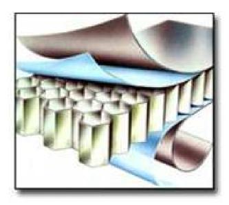
**Falconboard** is a rigid substrate made from a recycled paper honeycomb core with laminated paper facings of various paper grades to suit application and performance requirements. Recycled paper fibre content of Falconboard ranges from 25% for Mount and Print variants, to 95% for the Build version.
