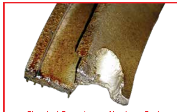
Chemical Corrosion on Aluminum Seal
