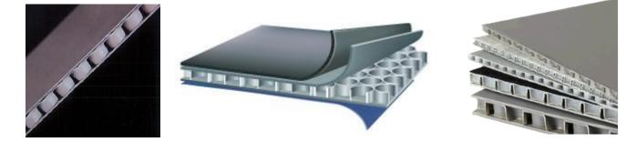
Bubble-X<sup>TM</sup> is a co-extruded PP sheet / air-bubble co-extruded PP film. A new patented technology, it is a co-extruded board made of three layers: a central thermoformed core, and two flat and compact "external skins" with "matte" finish. These external layers are smooth and corona-treated to reach outstanding printing performances.
